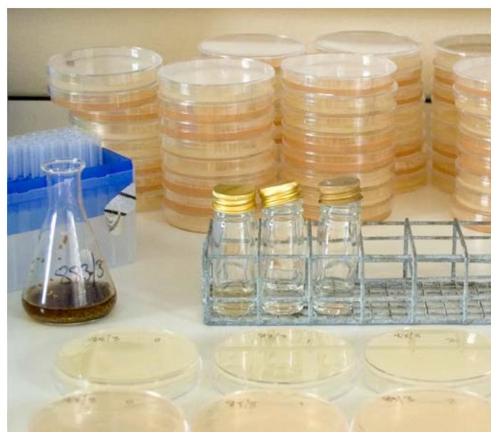
Figure 3. Seed testing for bacterial pathogens - dilution and plating
