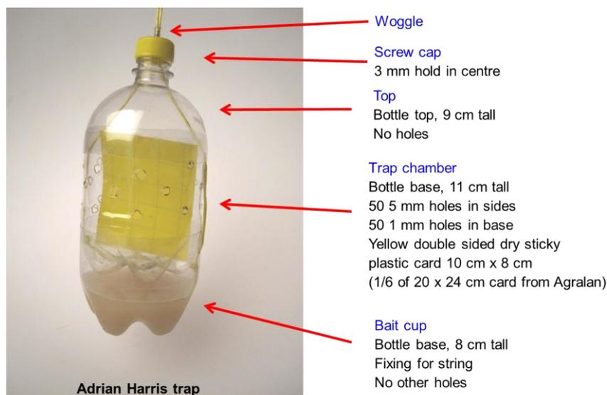
**Figure. Adult SWD monitoring trap designed by Adrian Harris, East Malling Research. The trap's unique and important design feature is the separate trap chamber where the sticky card is held. This design prevents adults from entering the liquid bait and also ensures that the card does not become contaminated with bait.**
