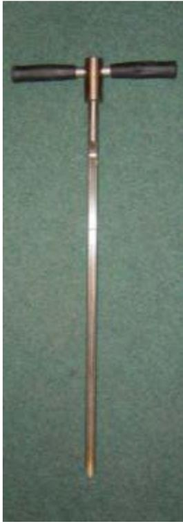
**Figure 2.** Lishman hammerhead core auger used to sample soil at three soil depths.
