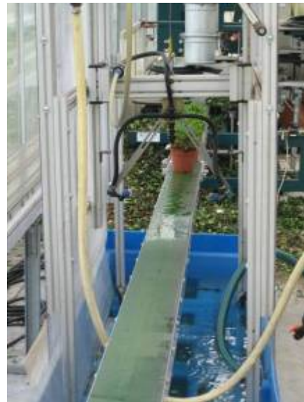
Figure 12. Spray cabin, made by Degramec Ltd in Belgium
