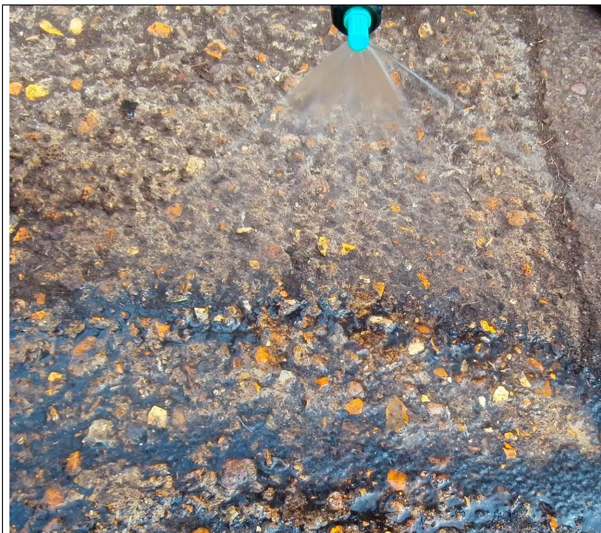
Figure 10: Worn deflector nozzle delivering a fingered spray patten
